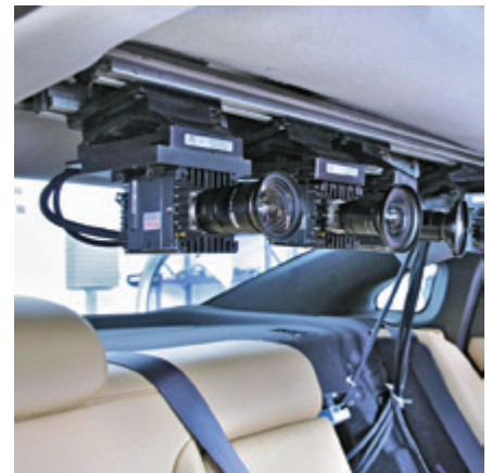
Phantom Miro C320J cameras installed on-board for a crash test
