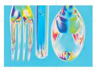
Image using AoLP data from DZK 33 UX250 and HSV color mapping visualizes residual stress in plastics and glass (birefringence).
