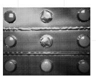
Standard visible-light intensity image of pills in blister pack. Glare and low contrast make presence detection difficult.
