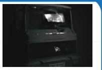
Image from DZK 33UX250: DoLP image data to reduce glare, making inside-view of cabin possible.
