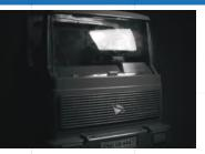
Standard visible-light intensity image with glare on windshield obstructing view inside.
